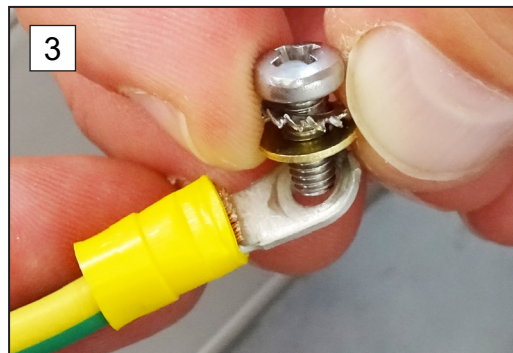
3. When assembling the potential equalization, pay attention to the correct order of serrated washer and flat washer: Screw head → serrated washer → flat washer → cable lug.
