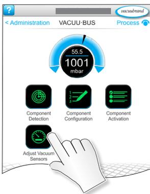
1. Evacuate the vacuum sensor to a pressure  $< 10^{-3}$  mbar.
