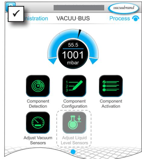
The buttons retrieve context menus. The context menus facilitate the use of presets for **VACUU-BUS** components (e.g., address configuration, detection of connected components). Vacuum sensors and level sensors, amongst others, can be calibrated in this sub-menu.
