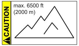
If the pump is installed at an altitude of more than 6500 ft (2000 m) above mean sea level, check compatibility with applicable safety requirements, and adopt suitable measures. There is a risk of the motor overheating due to insufficient cooling.
