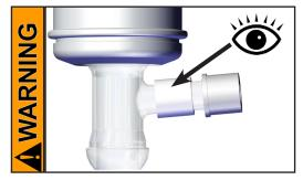
Check the overpressure safety relief device at the exhaust waste vapor condenser regularly; replace if necessary. Check especially for deterioration, coalescence and cracks.
