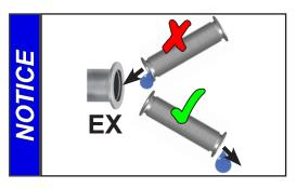
Always install outlet tubing descending from the pump or provide other measures to avoid backflow of condensate towards the pump.
