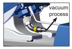
Connect the vacuum connection of the controller (measurement connection at the rear of the CVC 3000; hose nozzle for tubing I.D. 1/4" / 3/8" (6 / 10 mm) or connection for PTFE tube I.D. 3/8", O.D. 5/16" (10 / 8 mm)) via hose or PTFE tubing to the vacuum application. The cross-section of the tubing should be as large as possible.
