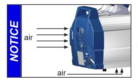
Make sure the fans' air supply is adequate. Do not place the pump on soft surfaces (e.g., rubber foam) during operation. This may reduce the air circulation in the pump housing and affect the fans' cooling effect. Check fans regularly for dust/dirt. Clean fan guard grills if necessary to avoid a reduction of ventilation.
