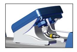
The CVC 3000 controller is equipped with an internal capacitive pressure transducer with ceramic diaphragm. It measures the actual pressure independently of the gas type, and with reference to the vacuum, i.e., absolute.
