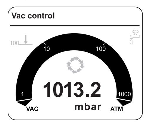
**Selected function** (displayed in the upper left corner): (A "function" is an operation mode of the CVC 3000 controller.)
