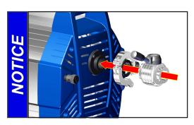
Use a suitable valve (see "Accessories / Spare parts", pg. 99) to isolate the pump from the vacuum application. This is to allow the pump to warm up before pumping condensable vapors and to clean the pump after use before it is switched off.
