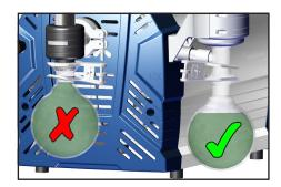
In case of **condensation**: Check the liquid level in the catchpots during operation. Check the liquid level in both catchpots regularly. Do not allow the catchpots to overfill. Drain catchpots in time to avoid overflow. Install a level sensor (see "Accessories / Spare parts", pg. 99) for monitoring, if necessary.
