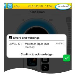
The triggering of the level sensor does not cause a process stop at once. The process continues to run until the **delay time** (adjustable at the controller) has elapsed.
