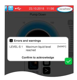
The delay time has elapsed. The process is stopped. Risk of overflowing catchpot.
